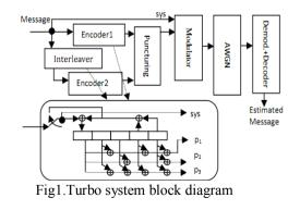
The original k information bits before input to the second encoder. The turbo codeblock is terminated by running each encoder for an additional K-1 bit times beyond the end of the information bit frame. Turbo code considered here has the following specifications [1]:
