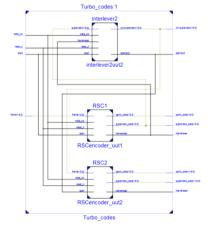
Fig5 RTL Turbo encoder based on the CCSDS Standard
