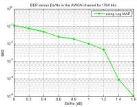
Fig4 BER performance of the CCSDS compliant turbo decoder in AWGN Channel
